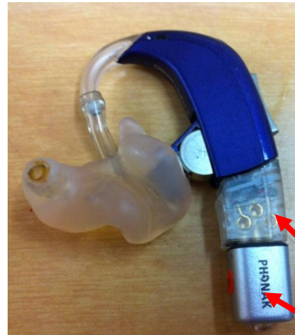
Phonak Extra Hearing Aid hearing aid with FM receiver attached
