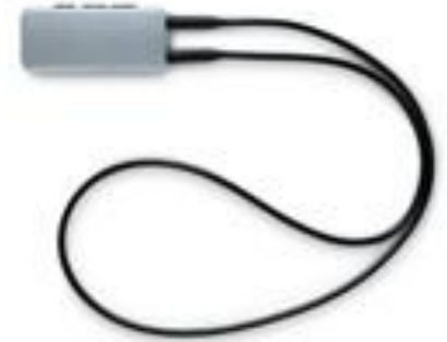
MyLink Neckloop receiver worn with a hearing aid or CI (works with a hearing aid's or CI's telecoil setting)
