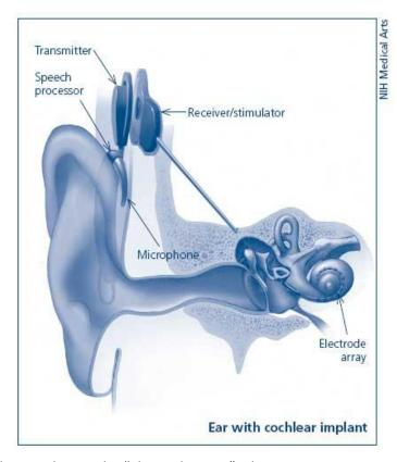
the sounds into electric impulses and then delivers the impulses to the "electrode array". The array recognizes the electric impulses and then sends this representation of sound through the auditory nerve to the brain so it can be interpreted and understood. A cochlear implant does not restore normal hearing. It provides representation of sounds in the environment and makes them available for the brain to interpret.
